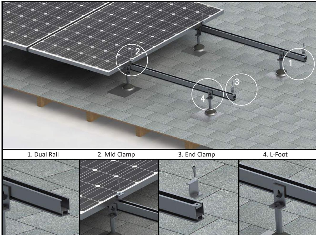
Figure 5. Exploded view of a flush mount installation with L-Foot
