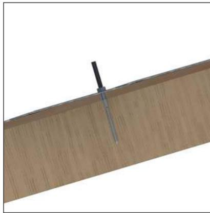
2. Insert the lag bolt through the 1.5" washer and 1.5" EPDM. Screw the 5/16" lag bolt into rafter, embedded min. 2.5".
