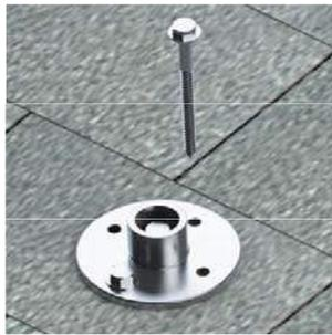
2. & 3. Screw the 5/16" lag bolt into the rafter, embedded minimum 2.5". Tightening torque is dependent on the roofing material.
