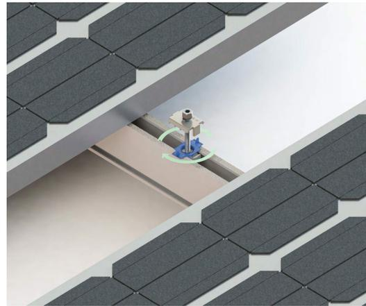
2- Lock the Channel Strut in the Dual Rack Rail channel by turning the Channel Strut Floater 180 degrees, which will ensure the grooves on the Channel Strut will line up with the lip of the Dual Rack Rail channel.
