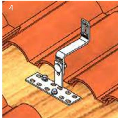
4. Attach the tile hook to the rafter using the three (3/16") or two (5/16") lag bolts, embedded a min. of 2.5"
