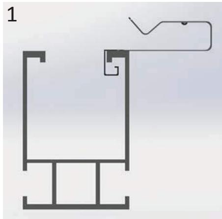
1. Place the cable clip on one of the Dual rail sides making a 90° angle.
