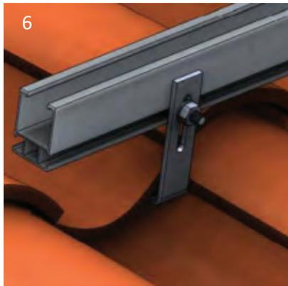
6. Attach the rail to the tile using 3/8" bolts, washer & nut. (Recommended: place star washer between the rail & S-tile adjustable hook).
