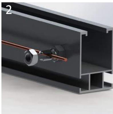
2. Tightening the grounding lug to (7ft. lbs) make sure the back plate teeth is biting the rail.
