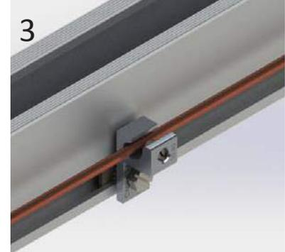
3. Push the grounding conductor (ground wire to be at minimum 10Ga) all the way to the back of the U-shaped slot and tighten the screw to (3 ft. lbs).
