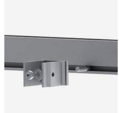
3. Slide the 3/8" bolt through the back side channel of the rail and attach to the U-bracket. Place one star washer between the rail and U-bracket.
