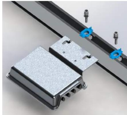
2. Lower or slide the channel strut through the Dual rail gap.
