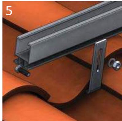
5. Slide the 3/8" bolt through the rail groove.
