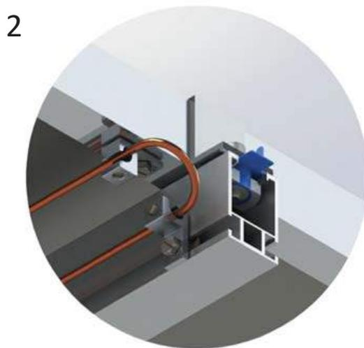
3. At the end of the string, bond both the last module and rail to the equipment grounding conductor, complying with electrical code.
