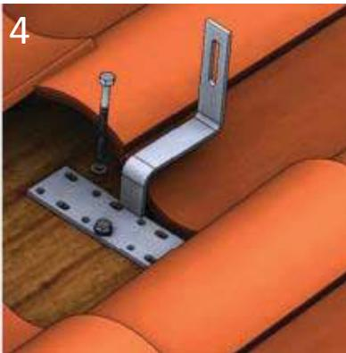
4. Attach the roof hooks to the rafter using the three (3/16") or two (5/16") hex bolts, embedded a minimum 2.5".
