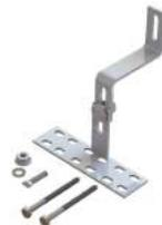
**14. Adjustable S Tile hook** - Use to mount rails on Spanish tile roofs. Adjustable upper arm enables variety of height to fit different sizes of Spanish tiles.
