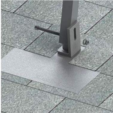
1. Attach the extension bar to the flash L-base using the M8 bolt, nut and star washer. Place star washer between the extension bar and L-foot.
