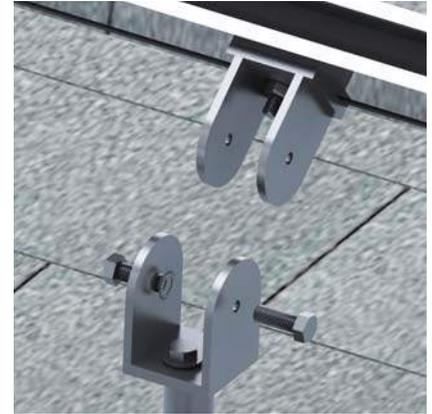
3. Align the angle bracket hole and secure it with the bolt and star washer, as shown above. (Tightening torque 14 ft.lbs).
