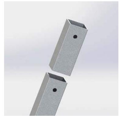
3. If the extension bar is longer than required, cut the extension bar and drill a hole using a 1/4" drill bit 0.8" below the cut line.
