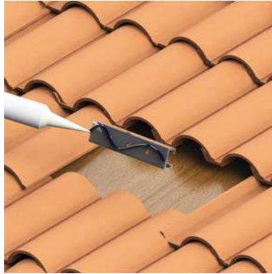
2. & 3. Insert the lag bolt through the tile strut base and apply compatible sealant.
