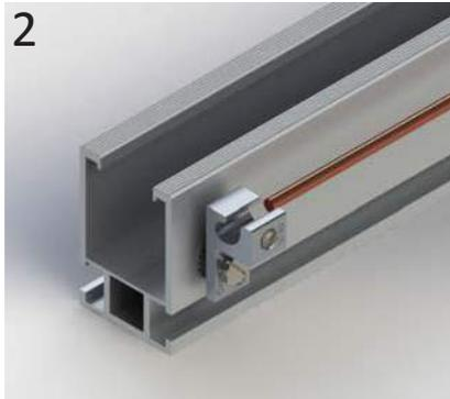
2. Tighten the grounding lug to (7 ft. lbs). Make sure the back plate teeth are biting the rail.
