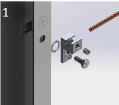
1. Slide the grounding lug through the module's grounding hole and attach to the back plate. (Tightening torque 7 ft. lbs). Make sure the back plate teeth are biting the module frame.
