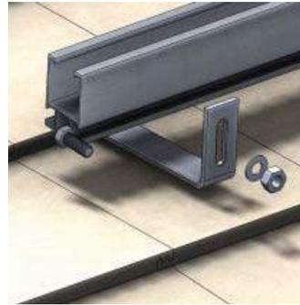
6. Slide the 3/8" bolt through the rail groove.
