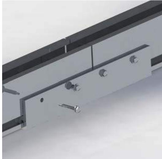
3. Tighten the first self-tapping screw all the way into the rail and tightening the rest until they just contract the rail, leaving it just loose enough for the rail to expand and contract within the splice. For rigid joint screw all the self tapping screws all the way into the rail. The choice between thermal expansion or rigid joints depends on the installation area.
