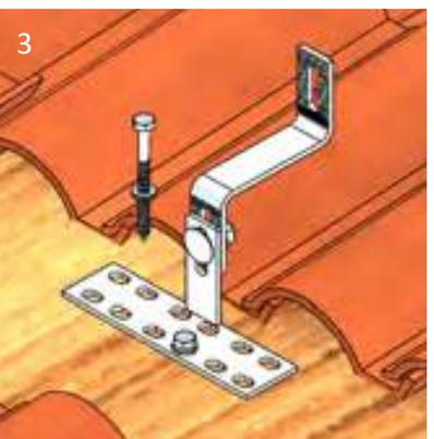
3. Insert the three (3/16") or two (5/16") bolts through the washer and S-tile hook, and apply fresh compatible sealant to the base. Tightening torque is dependent on the roof material. Adjust S-Tile hook height accordingly. Tighten the M8 flange nut.
