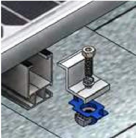
1. Insert the M8 allen bolt through the End clamp and screw the bottom to the channel strut.
