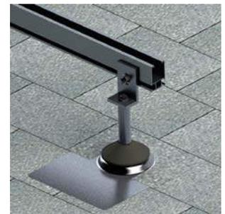
7. & 8. Attach the rail to the standoff using the top down or L-foot method. Please refer to page [3.4.1] & [3.4.2] for details regarding the rail to standoff attachment method. ( Do not exceed maximum torque value or you will damage the base).
