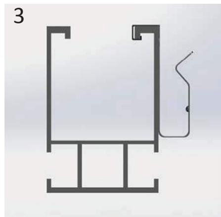
3. Make sure the cable clip is secured in place.
