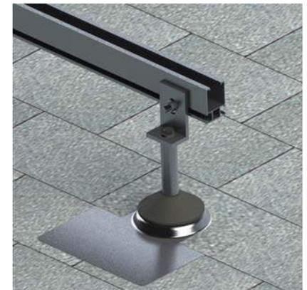
6. Attach the rail to the L-foot using a 3/8" bolt, star washer and nut. Recommended Torque 14 (ft. lbs.).
