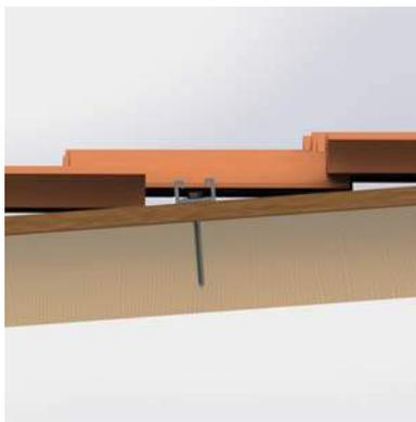
4. Screw the 5/16" lag bolt into rafter, embedded a minimum 2.5". Tightening torque is dependent on the roof material.
