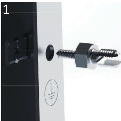
1. Slide the grounding lug through the modules grounding hole and attach to the back plate. Tightening tourq (7 ft. lbs) make sure the back plate teeth is biting the module frame.
