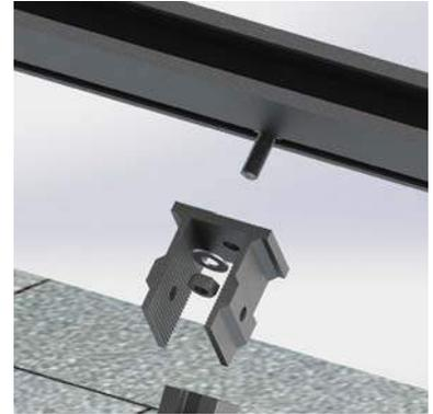
3. Slide the 3/8" bolt through the back side channel of the rail and attach to the upper leg base. Place one star washer between the rail and upper U-bracket
