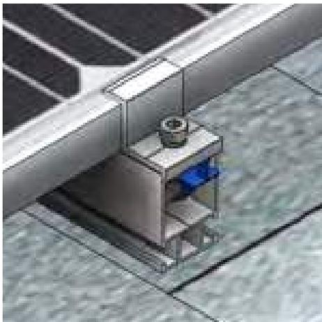
3. & 4. Screw the M8 bolt and the channel strut will align itself with the Dual rail grooves.
