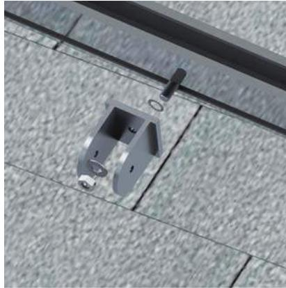
2. Slide the 3/8" bolt through the back side of channel of the rail and attach to the angle bracket. Place one star washer between the rail and angle bracket. (Tightening torque 14 ft.lbs ).
