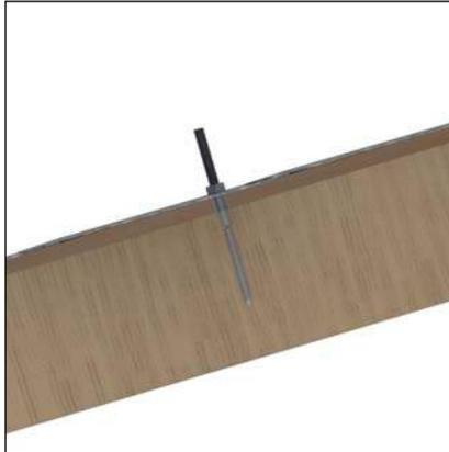
2. Screw the 5/16" lag bolt into rafter, embedded minimum 2.5". Tightening torque is dependent on the roofing material.
