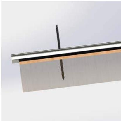
2. Screw the hanger bolt into the rafter, embedded a min. 2.5". Tightening torque is dependent on the roof material.
