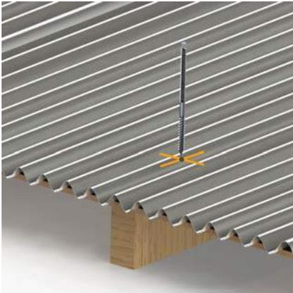
1. Drill a pilot hole using 5/16" drill bit through the roof material and into the center of the rafter at the planned location.
