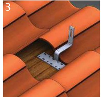
3. Position the roof hooks to the side of the underlying interlocking tile's valley.
