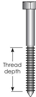
Use Table 6 to select a lag bolt size and embedment depth to satisfy your Uplift Point Load Force, R (lbs), requirements. Divide the uplift pointload by the withdrawal capacity, this results in inches of 5/16 lagbolt embedded thread depth needed to counteract the uplift force. If other than lag bolt is used (as with a concrete or steel), consult fastener mfr documentation.
