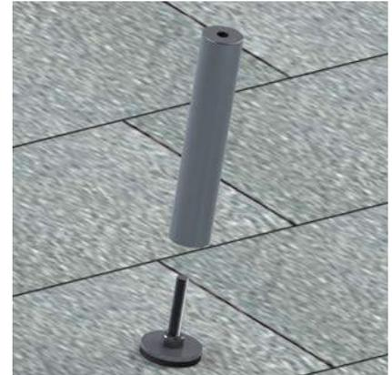
3. Install the EPDM and stainless steel washer and screw the standoff into the lag bolt.
