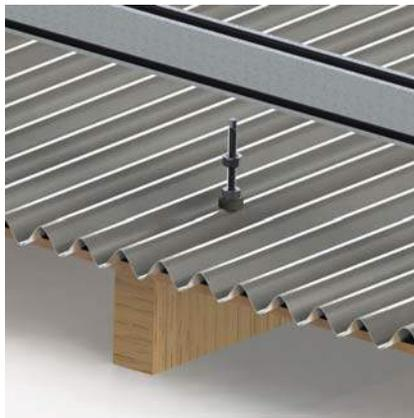
5. Drill a 3/8" hole through the rail for top down installation.
