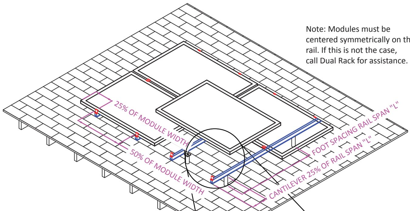
Note: Modules must be centered symmetrically on the rail. If this is not the case, call Dual Rack for assistance.
