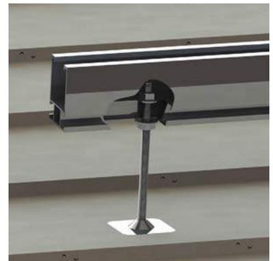
7. Use the two 3/8" nuts to engage the threaded headless bolt to the channel strut below the tile and remove the nut when done.
