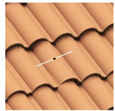
6. Carefully drill a hole through the tile using 1/2" drill bit.
