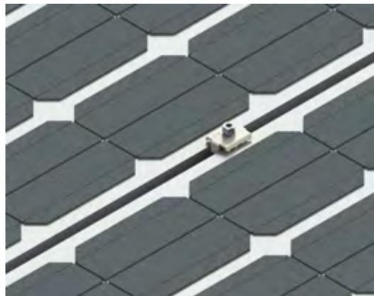
4- Make Sure the Grounding Mid Clamp teeth are “biting” center of the module frames to ensure electrical grounding continuity. Screw the M8 bolt (10 ft.-lb. torque recommended) and the Channel Strut will align itself with the Dual Rack Rail grooves.
