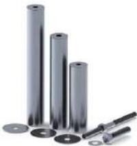
**7. Dual Jack (Standoff)** - Use Standoffs to increase the height of the array above the roof or to allow for the use of flashing. Use one per L-foot. Comes with 5/16" x 3.5" lag bolt, 3/8" x 1.5" flat washer and 3/8" x 1.5" rubber gasket, in mill finish or painted black.
