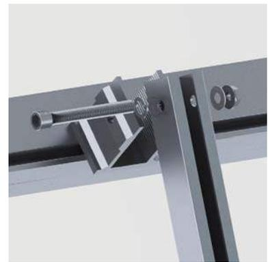
6. Secure the U-bracket to the extension bar using the M8 bolt, nut and star washer. Place star washer between the extension bar and U-Bracket.
