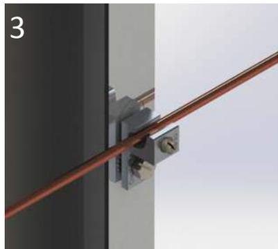
3. Tighten the screw to (3 ft. lbs).
