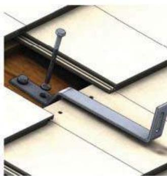
4. Attach the roof hook to the rafter using the two (3/16" or 5/16") hex bolts, embedded a minimum 2.5". Tightening torque is dependent on the roofing material.
