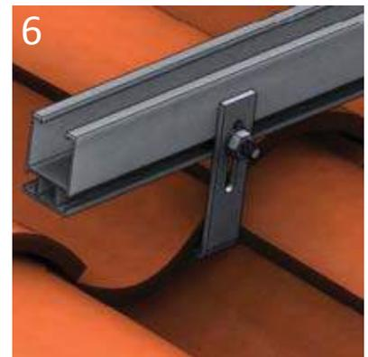
6. Attach the rail to the tile hook using 3/8" bolts and nut. (it's recommended to place the star washer between the rail and S-tile hook.)
