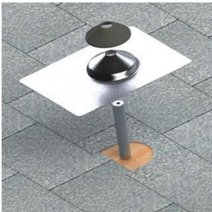
4. Install the flashing over the standoff and add the EPDM collar.
