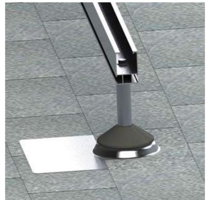
6. Screw the 3/8" bolt to the standoff. Recommended Torque 14 (ft. lbs.)
