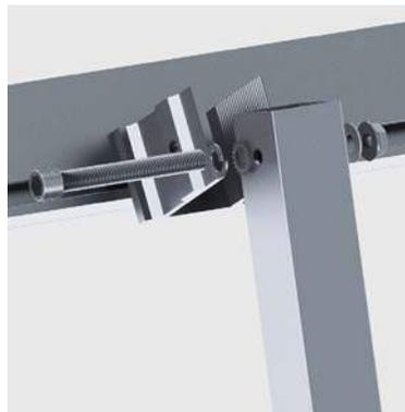
5. Secure the upper leg base to the extension bar using the M8 bolt, nut and star washer. Place star washer between the extension bar and U-bracket.
