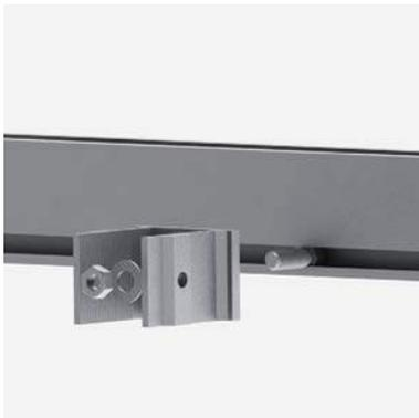
4. Slide the 3/8" bolt through the back side channel of the rail and attach to the upper leg base. Place one star washer between the rail and U-bracket
