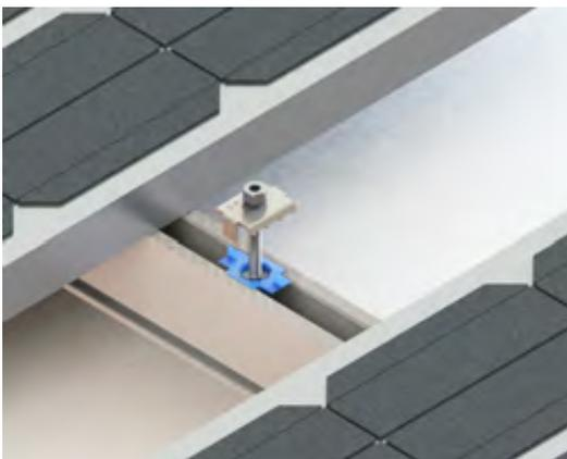
3- Verify that the Channel Strut is locked in the rail channel, using the Channel Strut Floater position (now parallel to rail channel) as a guide. Place the module(s) under the Grounding Mid Clamp, making sure the Grounding Mid Clamp teeth are in line with the module frame.
