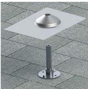
5. & 6. Install the flashing over the standoff and add the EPDM collar. Please refer to page [3.6] for detailed flashing installation.
