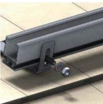
7. Attach the rail to the tile hook using 3/8" bolts and nut. (It's recommended to place a star washer between the rail and flat tile hook).
