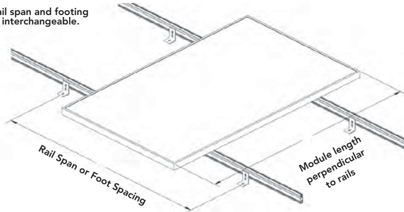
Note: Modules must be centered symmetrically on the rails (+/- 2\*), as shown.
