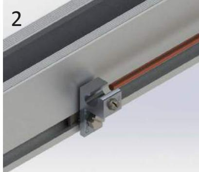
2. Tighten the grounding lug to (7 ft. lbs). Make sure the back plate teeth are biting the rail.
