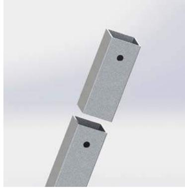
2. If the extension bar is longer than required, cut the extension bar and drill a hole using a 1/4" drill bit 0.8" below the cut line.
