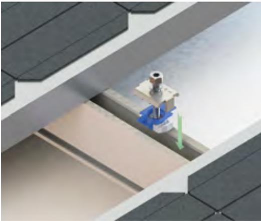
1- Insert the Grounding Mid Clamp Channel Strut in a parallel configuration into the Dual Rack Rail channel opening. The blue Channel Strut Floater will ensure that the Grounding Mid Clamp will be supported and stay in place for complete installation.
