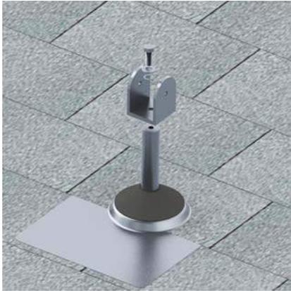
1. Attach the angle bracket to the standoff and secure it using the bolt. Make sure the order of the star washer and the flat washer is as shown above. Tightening torque (14 ft. lbs).
