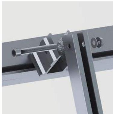
7. Secure the upper leg base to the extension bar using the M8 bolt, nut and star washer. Place star washer between extension bar and U-bracket.
