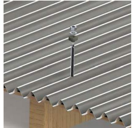
3. Place the EPDM, flat washer and nut and secure the bolt. (Tightening torque dependent on the roof material).
