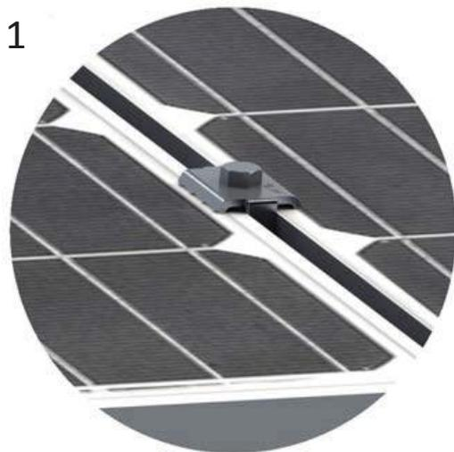
1. Grounding mid clamp electrically bonds the module's frames together. (Up to 44 modules per #6 bare copper wire.)
